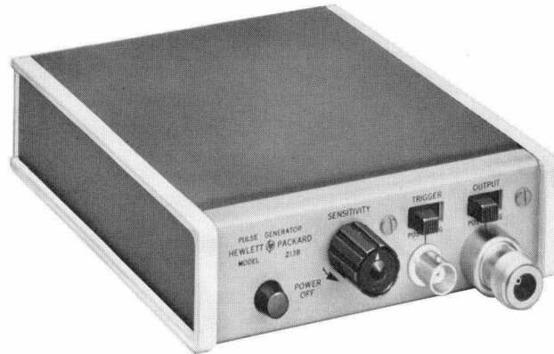
Fig. 1. Tunnel-diode pulse generator provides voltage steps with 0.1 nanosecond risetime for testing very fast systems. Repetition rate can be up to 100 kc.
